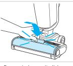
**5.** Reinstall brush roll window. Align tabs on edges of foot.
